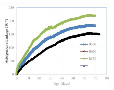
Figure 4. Effect of unit quantity of binder on autogenous shrinkage
