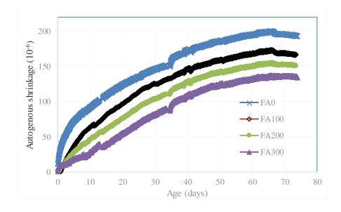
Figure 3. Effect of fly ash content on autogenous shrinkage
