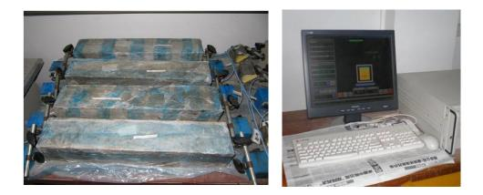
(a) Stereogram of the test setup(b) Data acquisition systemFigure 2. Test setup of autogenous shrinkage of self-compacting concrete
