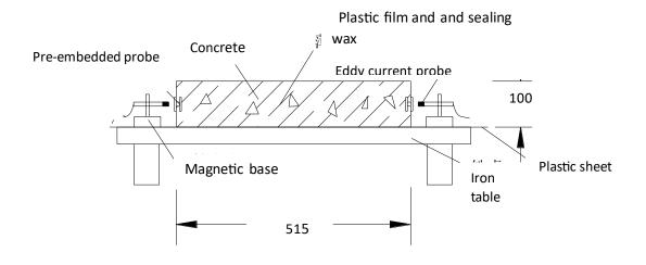
Figure1. Schematic view of autogenous shrinkage test setup (unit: mm)
