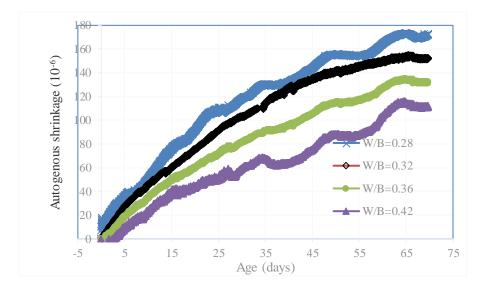
Figure 5. Effect of water-binder ratio on autogenous shrinkage
