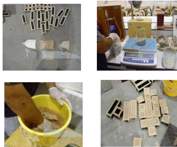
Figure 4: Steps to use to produce the new mortar
