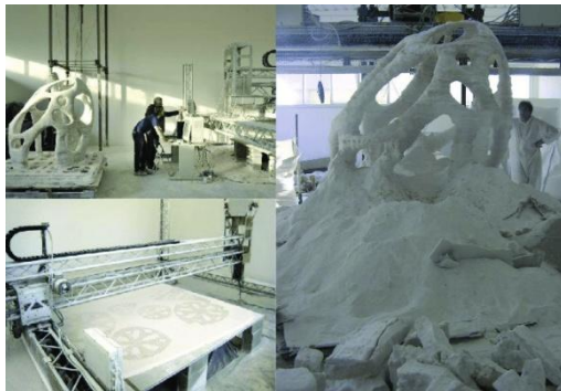
Figure 5 : an example of D-Shape 3D Printing Technology
