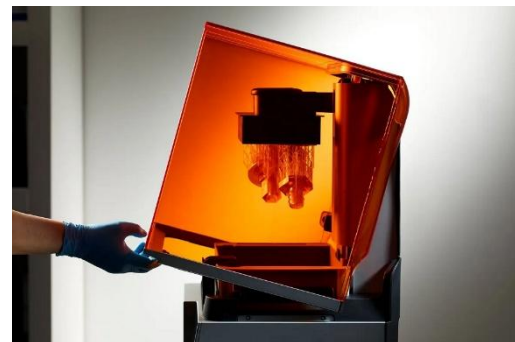
Figure 4 : a new example of Stereolithography (SLA) 3D Printer In its contemporary form
