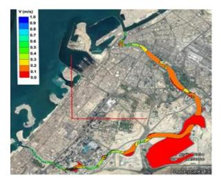
figure 4. Water velocity behavior in Dubai Creek and Canal [8]
